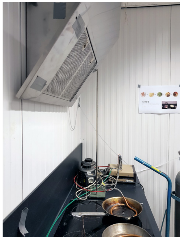
Figure 4. Laboratory setup for cooking: left chimney hood with 95% coverage of front burners, right slanted hood with 0% coverage of front burners.
