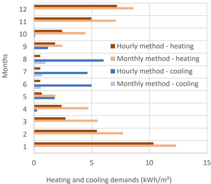
Figure 7. Comparison of energy requirements in kWh/m<sup>2</sup> per year calculated by monthly and hourly method. The figure shows not only the lower energy demand calculated by the hourly step, but also the cooling demand in April, May, September, which remained hidden using the monthly method.
