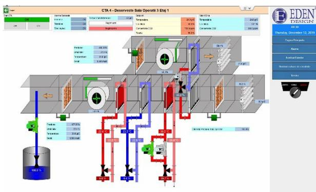
Figure 6. BMS – CTA 4 control panel.
