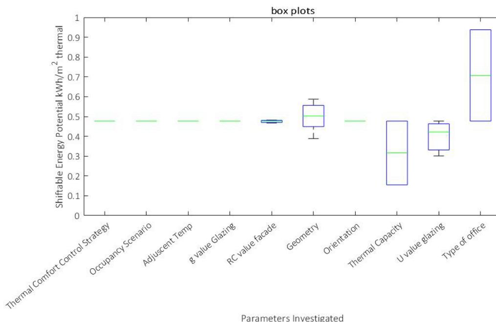
**Figure 8.** Box plots for each building variation investigated; each box shows the performance variation that is expected when changing the corresponding building parameter within defined ranges – Shiftable Energy Potential.
