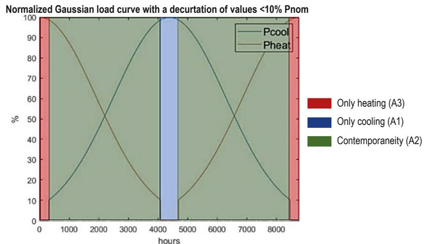
**Figure 2.** Example of Gaussian load curves.
