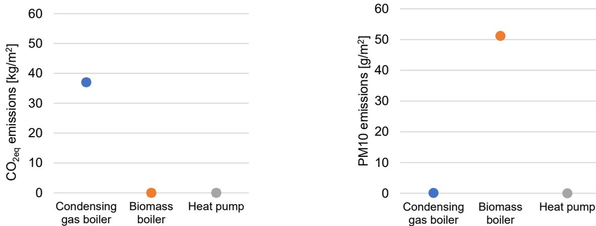
**Figure 2.** Environmental performances (in terms of direct emissions) of the technological options for MFH < 1980 North-West – space heating: a. CO<sub>2eq</sub> emissions; b. PM10 emissions.
