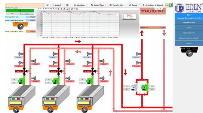
Figure 7. BMS – control panel of heating plant.
