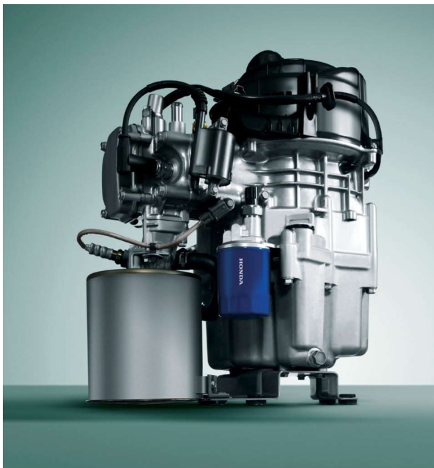
Figure 4. Gas-Internal Combustion Engine (single-cylinder four-stroke piston engine). Electrical output 1 kW with efficiency of 26.3%, thermal output 2.5 kW with efficiency of 65.7% and total efficiency of 92% (nett cv). Image source: www.Vaillant.com
