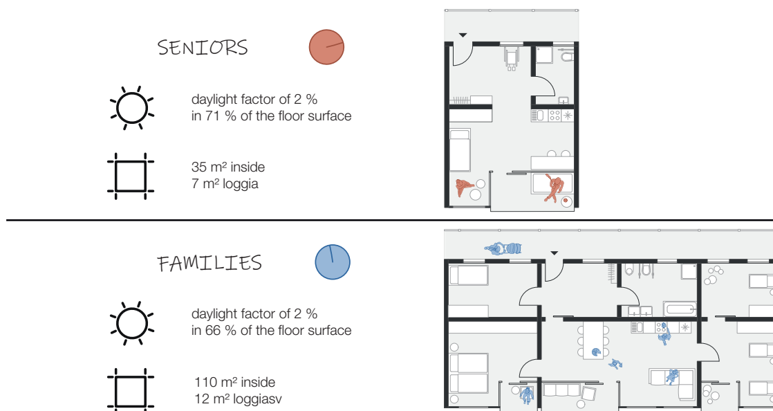
Figure 5. Detailed floor plans of two out of the four household types (seniors and families).
