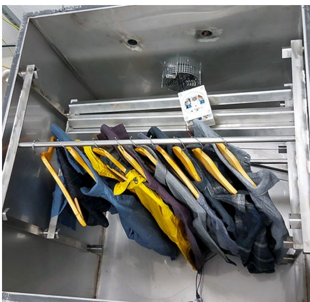
Figure 2. Positioning of the E-Nose and the product inside the emission chamber.
