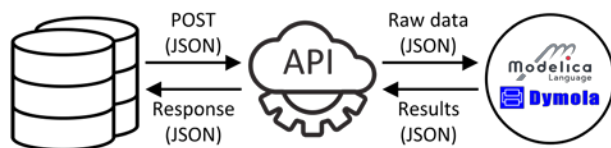
Figure 3. Interaction between the database and the toolchain through an API.
