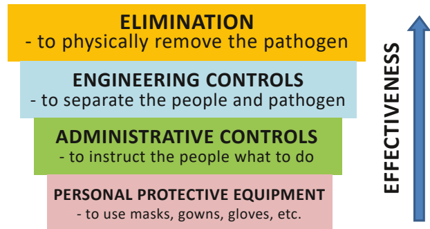
Figure 1. Hierarchical infection control pyramid, adopted from REHVA (2020), with four levels, for reducing the relative risk of airborne infection, where the top level is most effective and the bottom least effective.
