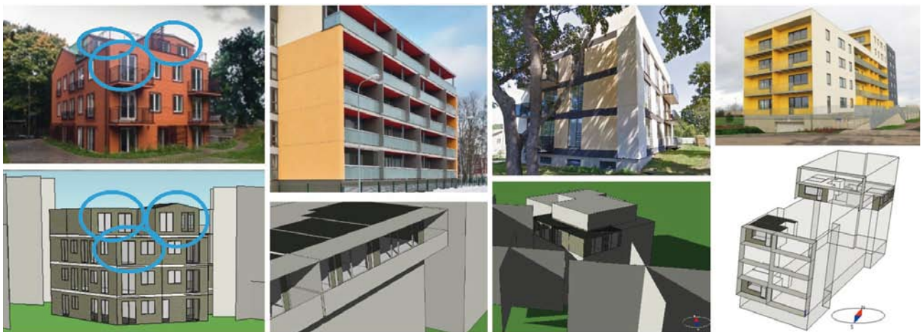
Figure 2. Rooms most likely to counter overheating are modeled and simulated. At least two 'critical' rooms – one bedroom and one living room must be analyzed in case of residential buildings.
