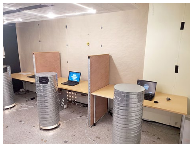
Figure 2. Climate chamber test layout. (Fan = table fan; Eva = evaporative cooling device; Jac = air-cooled jacket).
