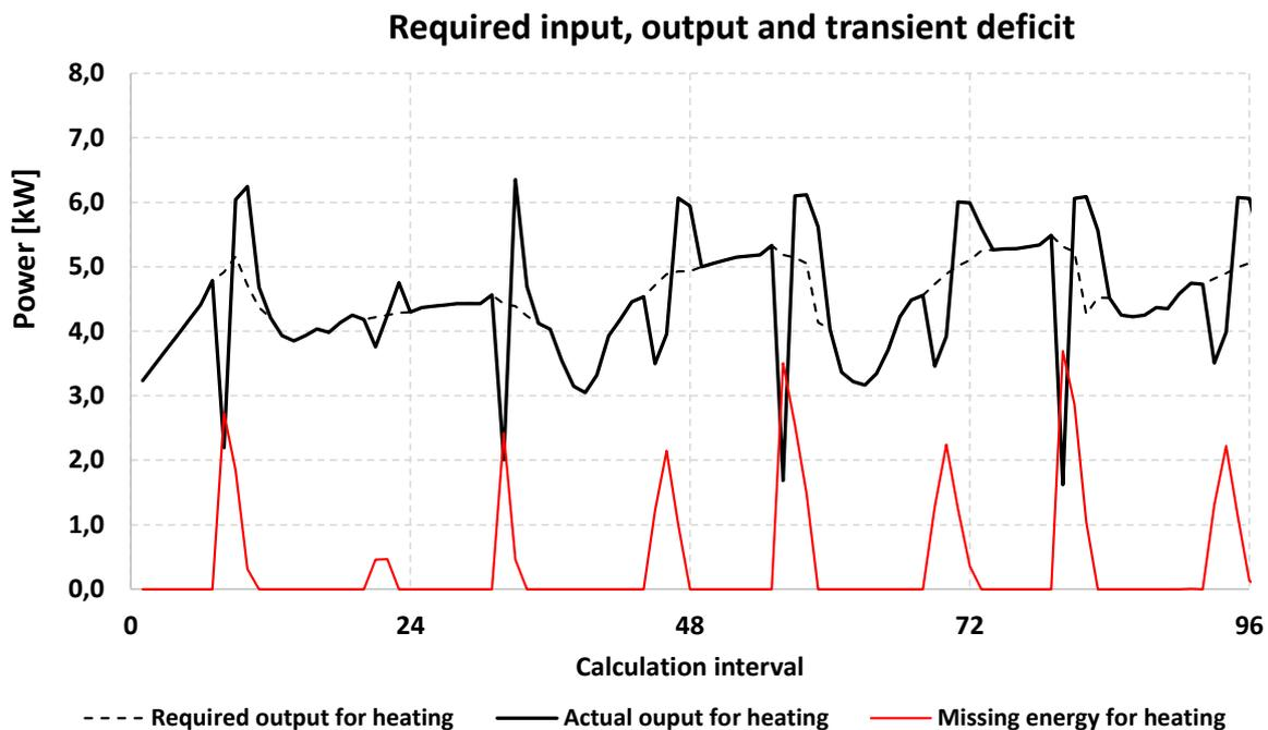
Figure 10. Example of transient heating power deficit.
