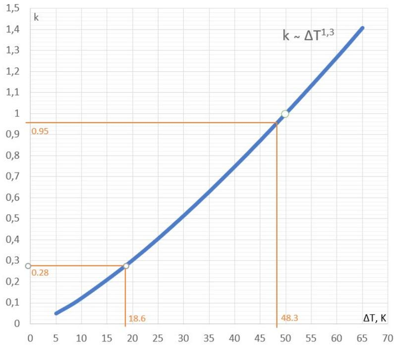
**Figure 3.** Dependence of radiator output ratio  $k$  on excess temperature  $\Delta T$ . For example, the radiator output at an excess temperature  $\Delta T$  18.6K ( $T_{flow}/T_{rtn}/T_{in} = 45/35/21^\circ\text{C}$ ) can be calculated using a diagram when the radiator output is known at another excess temperature, for example  $\Delta T$  48.3K (80/60/21 $^\circ\text{C}$ ) the output is 1000 W. New output is obtained:  $1000 \text{ W} \cdot 0.28/0.95 = 295 \text{ W}$ .
