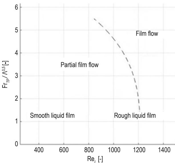
**Figure 6.** The proposed flow pattern map as a function of  $Fr_{TP}$ ,  $\Lambda$ , and  $Re_L$  for condensing ammonia inside a corrugated GPHE describing the transition from partial film flow to film flow.
