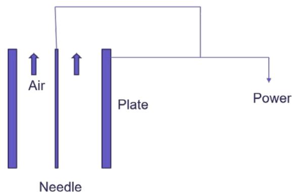
**Figure 3.** Schematic view of the corona discharge ioniser technology (Rahimi, 2013).
