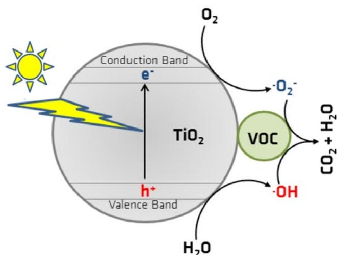
**Figure 2.** Schematic representation of photocatalytic oxidation of a volatile organic compound (VOC) (Mull et al., 2017).
