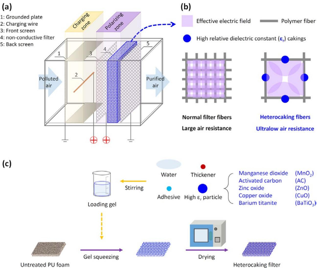
**Figure 4.** (a) Schematic of the electrostatically assisted heterocaking (EAHC) air filter module, (b) schematic of heterocaking (HC) fibres in a polarising field compared with standard filter fibres, and (c) preparation process of HC filters by a fast and large-scale roll-to-roll gel squeezing method. (Tian et al., 2020).
