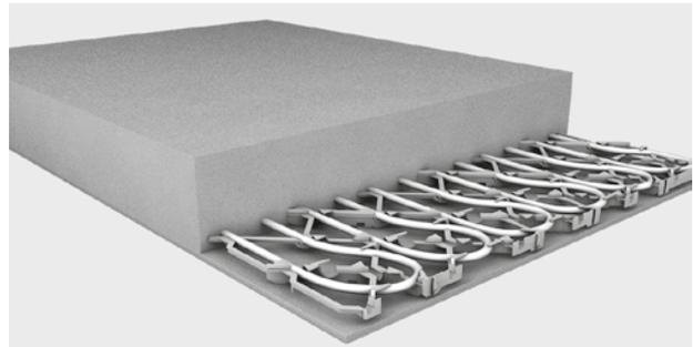
**Figure 4.** Thermally activate building systems like Uponor Contec ON are a very economical solution. They are integrated into the concrete ceiling during the construction of the building.
