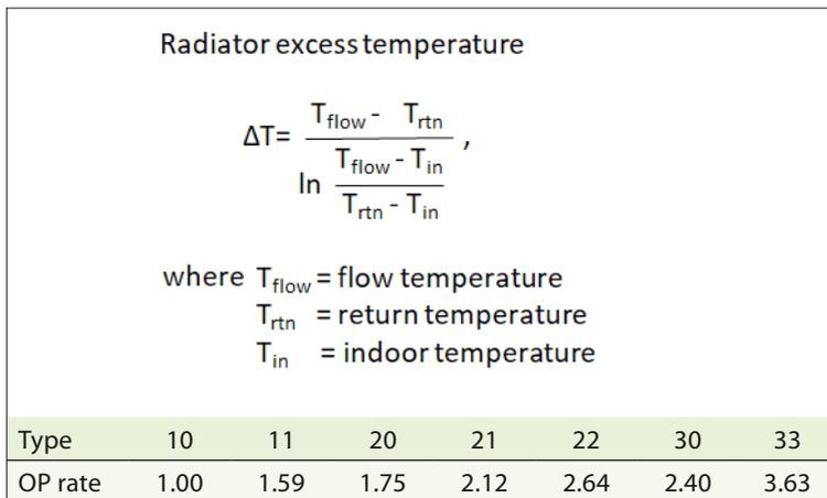
**Figure 4.** Output ratios of panel radiators according to radiator type. The type designation describes the number of panels and convection plates. For example, type 21 means that the radiator has two water circulating panels and in addition one convection plate. For example, the output of type 22 is  $2.64 / 1.59 = 1.67$  times higher than the output of type 11 at the same width / height dimensions.
