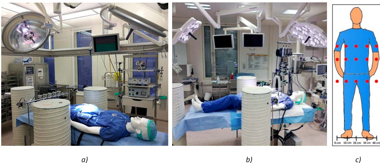
Figure 2. Experimental setup: a) photo of the operating room with a LAF; b) photo of the operating room with an MV; c) location of measurements. [4]
