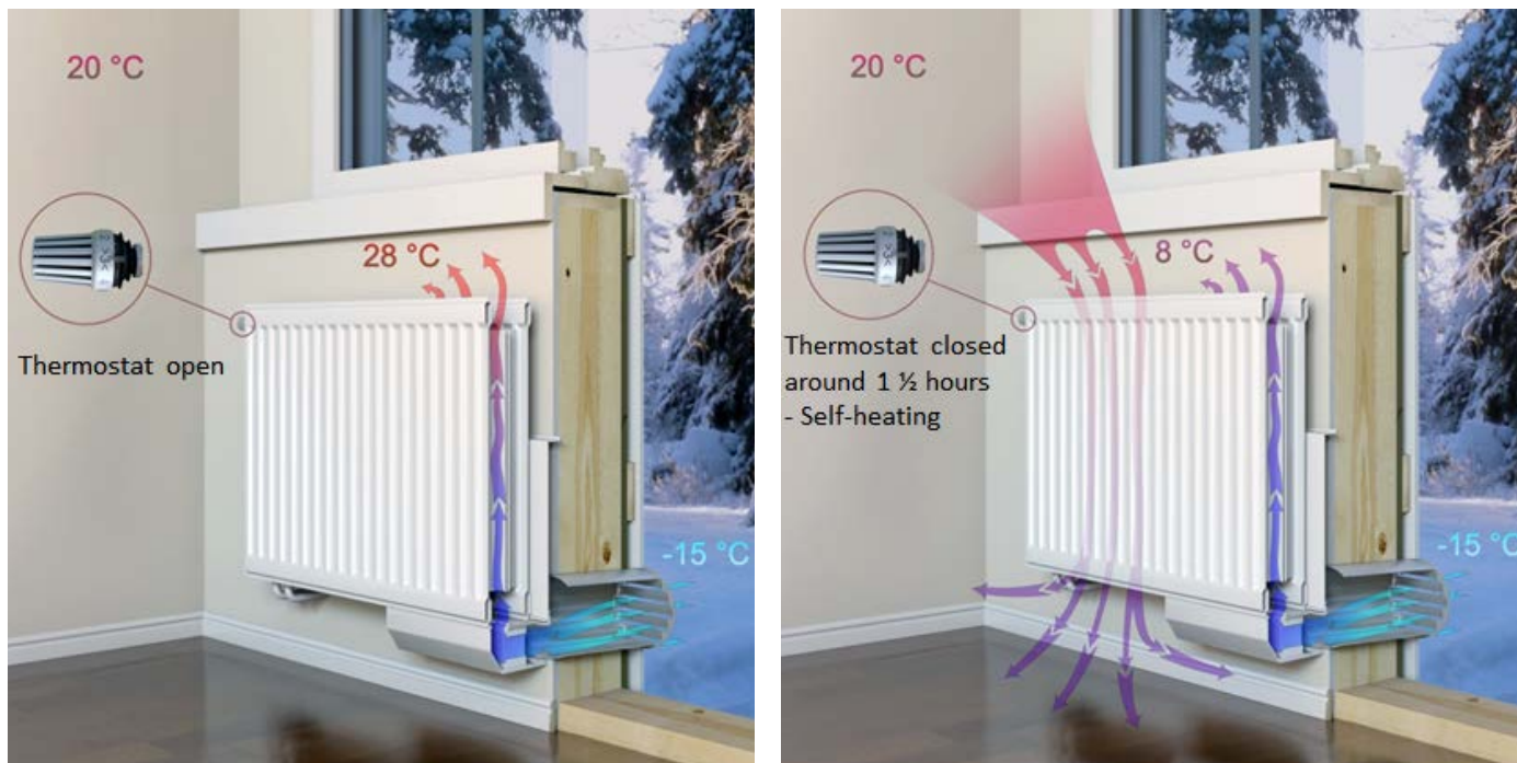
Figure 4. When the radiator temperature drops below room temperature the radiator starts to absorb heat from the room and the supply air warms up.
