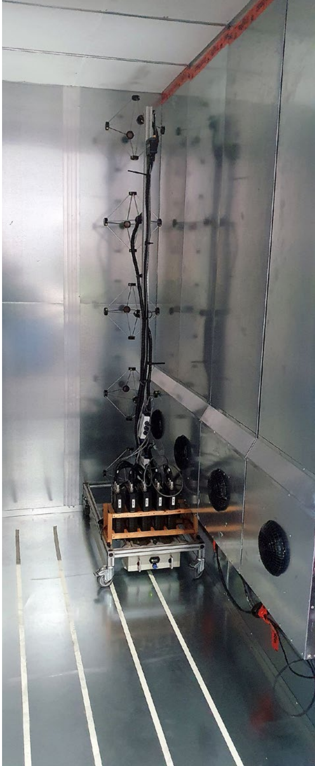
Figure 3. Test elevator cabin with setup for air velocity measurements. On the right side of the picture four centrifugal suction fans in the wall cavity are visible.
