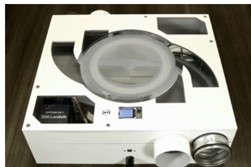
Figure 1. Concept of the Counterflow Heat Recovery Fan. Cross section of the flow conduction (top) [2] and manufactured laboratory prototype (bottom) [3]
