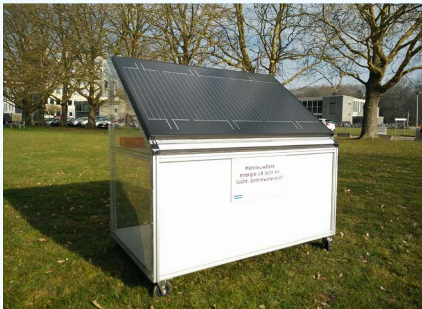
Bioscience engineers from KU Leuven have designed a solar panel that converts 15 percent of the sunlight straight into hydrogen gas – a world record. © Tom Bosserez
