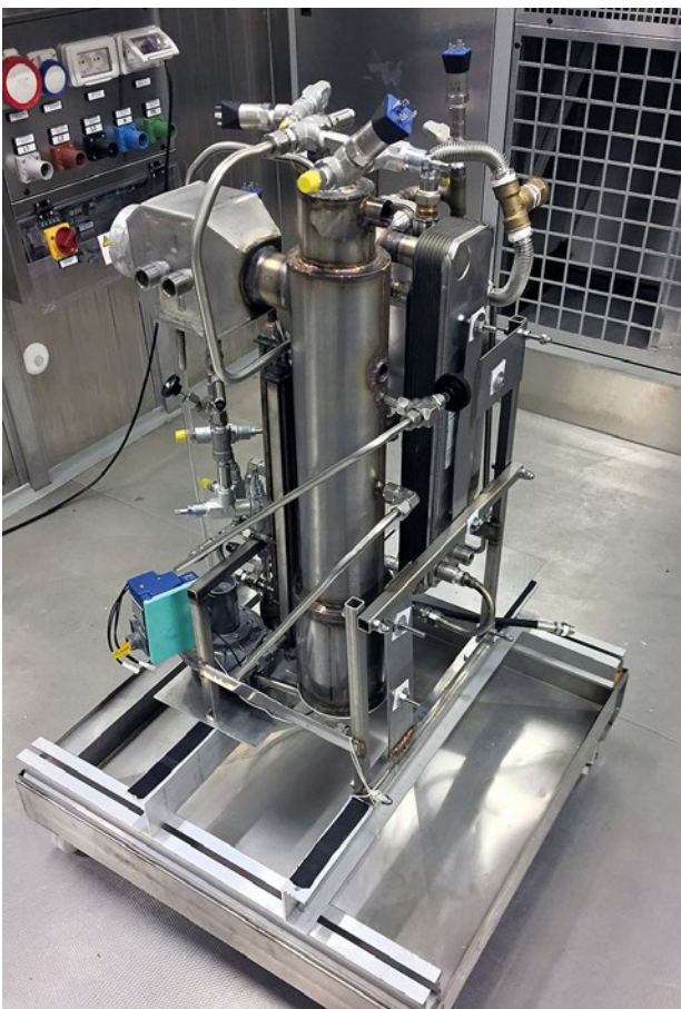
Figure 1. View of two sides of the GdAHP prototype, showing the assembly of components.
