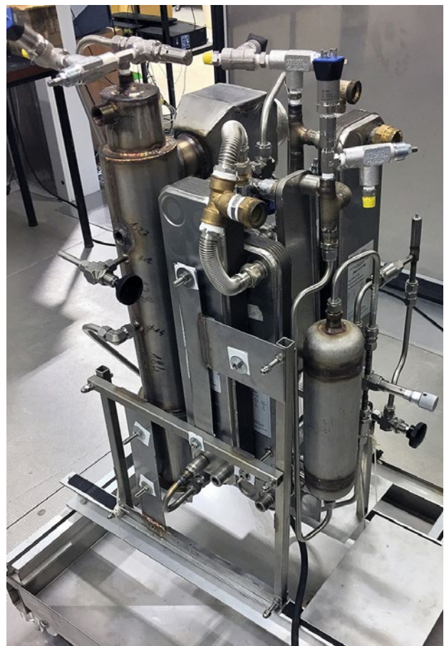
Figure 1. View of two sides of the GdAHP prototype, showing the assembly of components.
