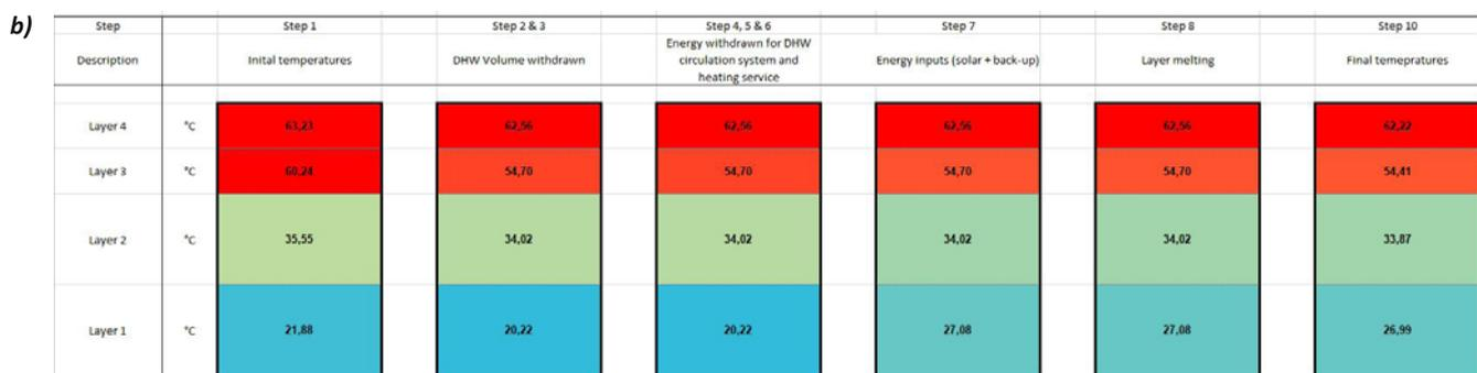
Figure 4. a) Storage tank temperatures in a chosen hour; b) Insight of each calculation step temperature stratification).
