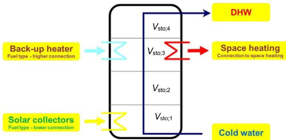
Figure 1. Graphical representation of a storage module mathematical model (Method A).
