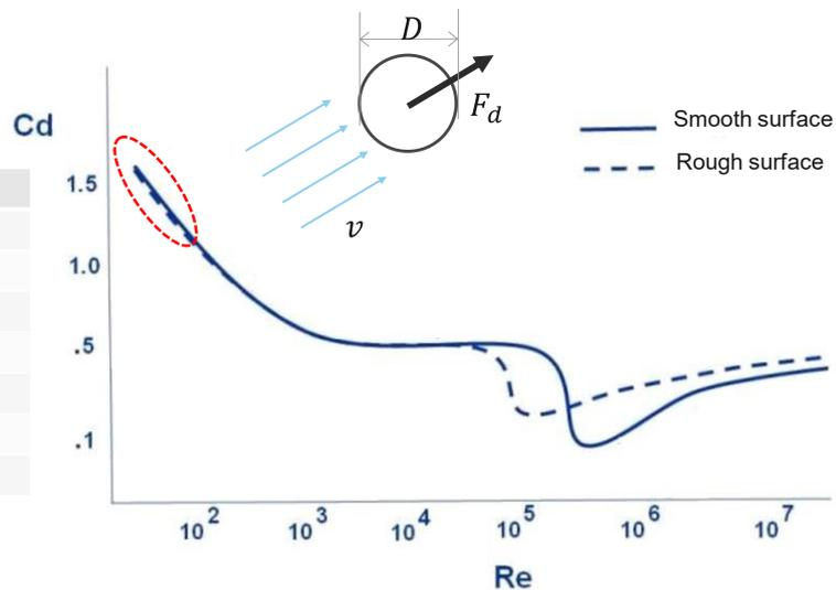
Figure 4. Aerodynamic resistance coefficient as a function of Reynolds Number for a sphere.
