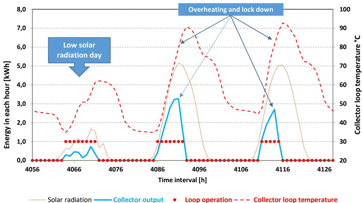
Figure 2. Identifying overheating and lock-down of collector loop.
