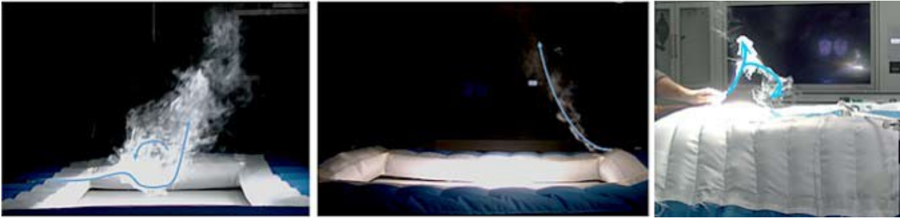
Figure 7. Smoke tests for the long and short side for the configuration 1 blanket (left, middle) and the short side for configuration 2 (right).
