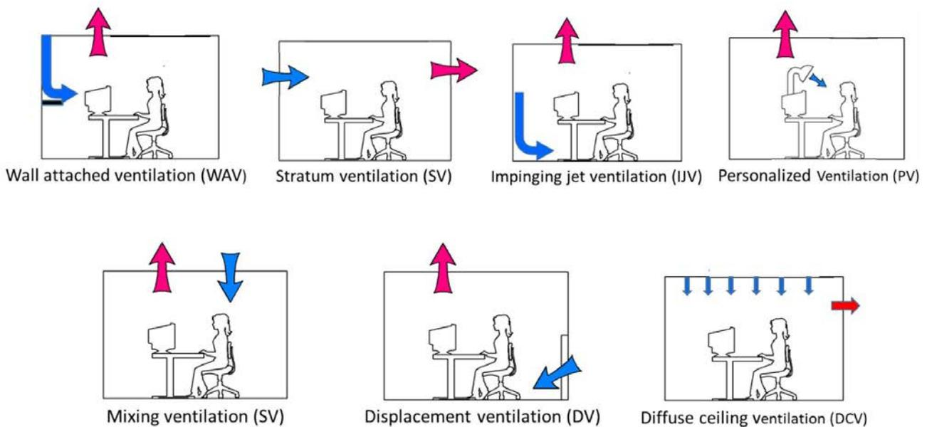
Figure 3. The simulated air distribution methods (blue arrows: supply; red arrows: exhaust).
