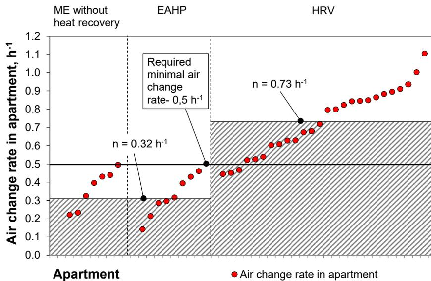
**Figure 2.** Air change rates measured in apartments renovated after 2015, with new ventilation requirements, in operation about one year after handing over.
