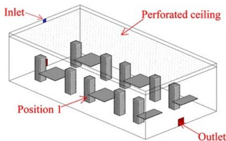
g) Diffuse ceiling ventilation (DCV) with perforated ceiling
