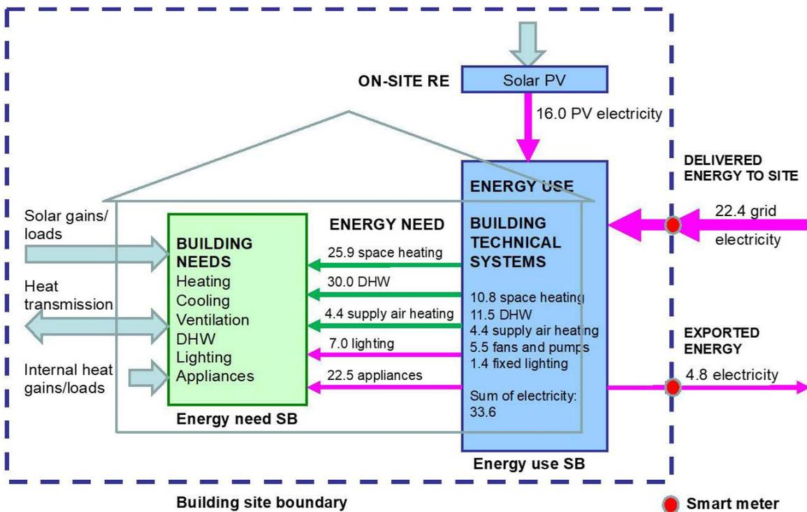
**Figure 2.** Energy flows for delivered and exported energy calculation. Note that internal heat gains (under energy needs) include the full lighting as well as appliances which are not included in EPB services but are used for PV self-use (otherwise PV self-use of 70% would be impossible).
