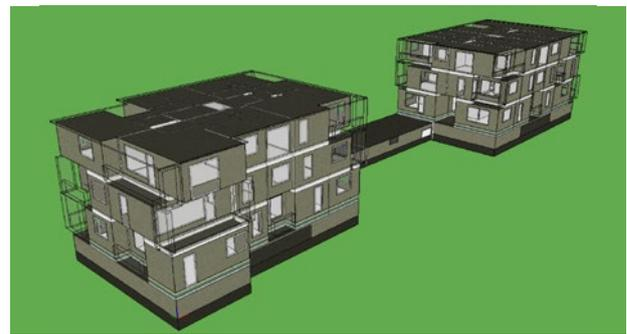
U<sub>wall</sub>=0.14; U<sub>roof</sub>=0.12; U<sub>floor</sub>=0.14; U<sub>window</sub>=0.9; q<sub>50</sub>=1.5 m<sup>3</sup>/hm<sup>2</sup>. Heat recovery ventilation, 80% temp.ratio, electric reheating coil. No cooling (passive measures to control summer thermal comfort). Heat source options: DH (district heating), Gas (gas boiler), GSHP (ground source heat pump) and AWHP (air to water heat pump).
