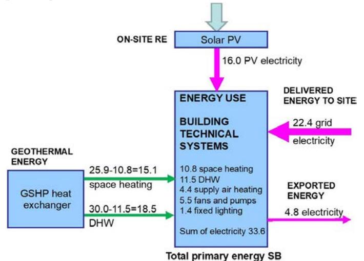
**Figure 3.** Energy flows for total primary energy calculation.
