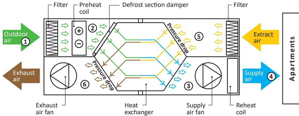
**Figure 1.** Principle sketch of residential AHU with counter flow heat exchanger:
