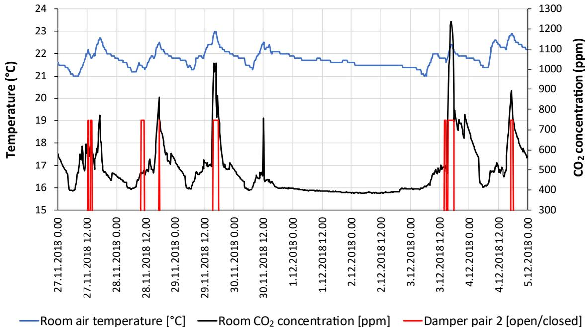
**Figure 1.** Performance of DCV system in Space 2.
