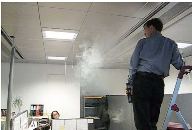
Figure 7. Flow visualization with smoke generator.
