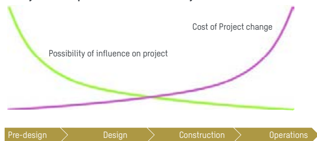
Figure 7. Deficiencies found when testing and monitoring the completed construction are usually costly to fix.
