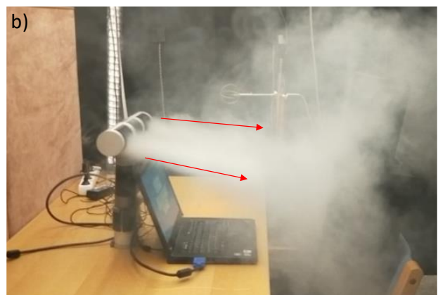
Figure 3. Smoke visualization of the personalized airflow pattern with PVRP system a) 7 l/s and b) 15 l/s. The red arrows show the main direction of the air jet.
