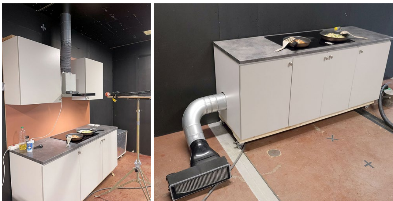
Figure 2. Ducted standard setup (left) and downdraft recirculating solution (right).
