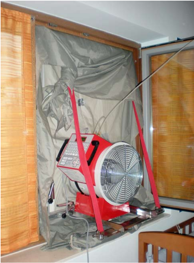
Figure 4. Blower Door test.
