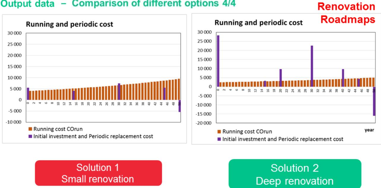
Figure 9. Example of comparison of the annual running and periodic replacement costs for different level of renovation
