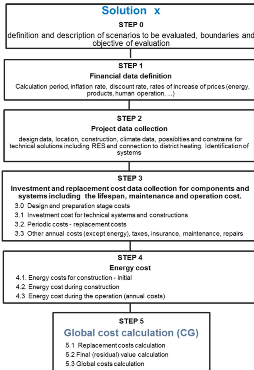
Figure 2. Example of flowchart for calculation of global costs.
