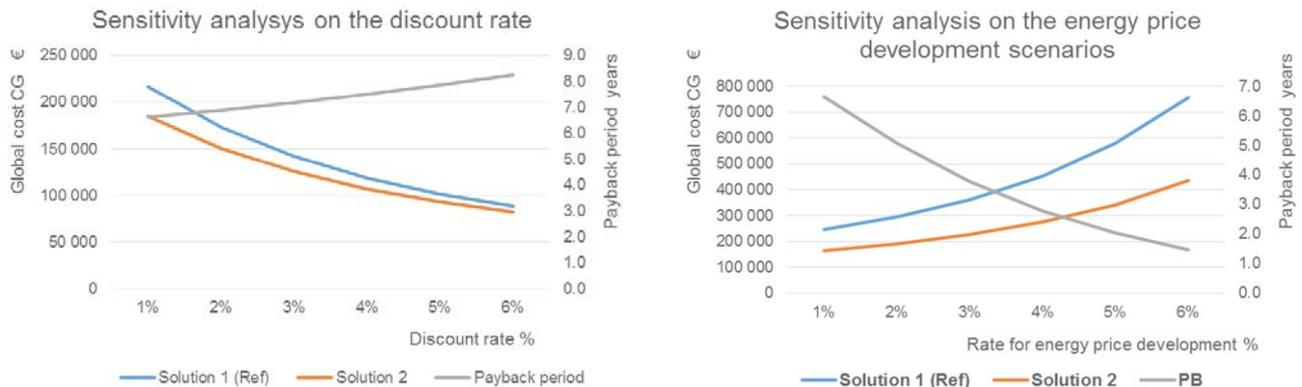
Figure 5. Example of sensitivity analysis on the most influencing parameters.
