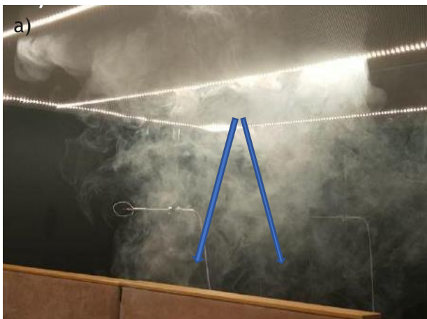
Figure 2. The smoke visualization of the low velocity system (LVRP) a) the local air distribution with the airflow rate of 10 l/s and b) the local air distribution with the airflow rate of 15 l/s. The blue arrows show the direction of the local airflow.
