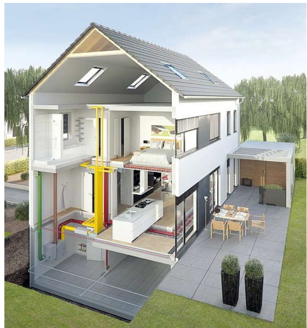
Figure 1. Representation of the ventilation system. Green: outdoor air; Red: supply air; Yellow: extract air; Brown: exhaust air; Grey: the ground collector with glycol-water mixture.
