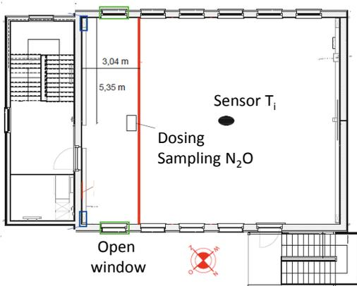
**Figure 5.** Test set up tracer gas measurement.
