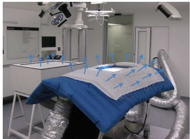
Figure 6. Full-scale test setup of the ventilating blanket and instrument table of configuration 1 (left) and configuration 2 (right) in the mock-up of the OT, the blue arrows indicate the clean airflows.
