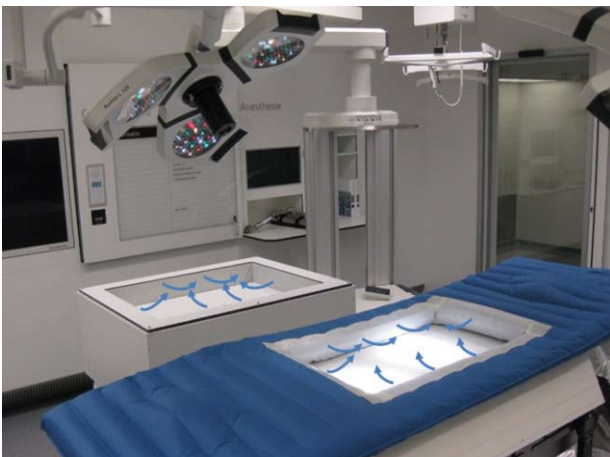
Figure 6. Full-scale test setup of the ventilating blanket and instrument table of configuration 1 (left) and configuration 2 (right) in the mock-up of the OT, the blue arrows indicate the clean airflows.
