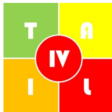
Figure 1. Graphical presentation of the TAIL rating scheme including four IEQ components: thermal environmental quality (T), the acoustic environmental quality (A), the indoor air quality (I), and the luminous (visual) environmental quality (L), as well as the overall IEQ in the centre.
