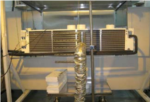
Figure 1. CO 2 evaporator testing.
