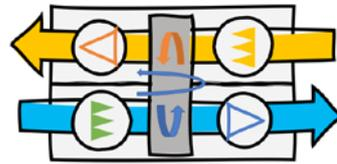
The fourth mode of leakage is from extract to supply on the room side of the rotor like this:
