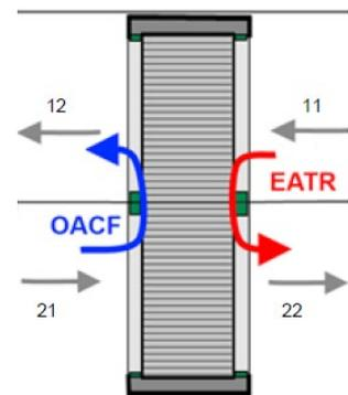
OACF is the ratio of the outdoor air inlet and the supply air outlet flow:
