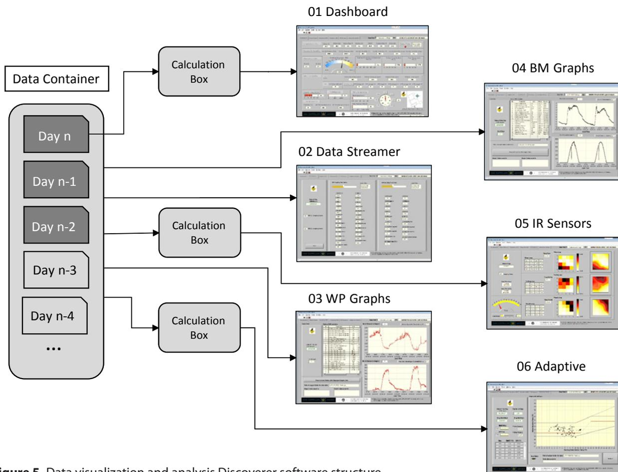
Figure 5. Data visualization and analysis Discoverer software structure.
