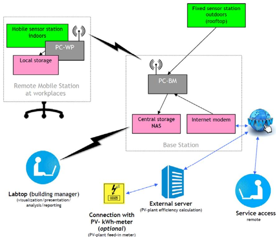
**Figure 2.** Architecture of the developed monitoring system.
