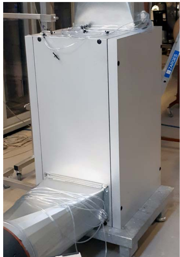
Figure 2. The NeGeV prototype PCM module with the CSM casings from Rubitherm inside.
