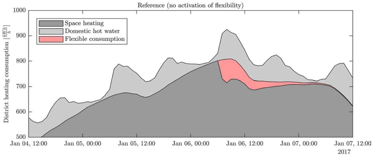
**Figure 4.** Simulated district heating consumption in the modelled 159 residential buildings. The models of building thermal dynamics and domestic hot water consumption are used to depict the consumption as the potentially flexible demand for space heating and the inflexible demand for preparation of domestic hot water. The red marking shows the part of the reference consumption that will be shifted in time in this example (see **Figure 3**).
