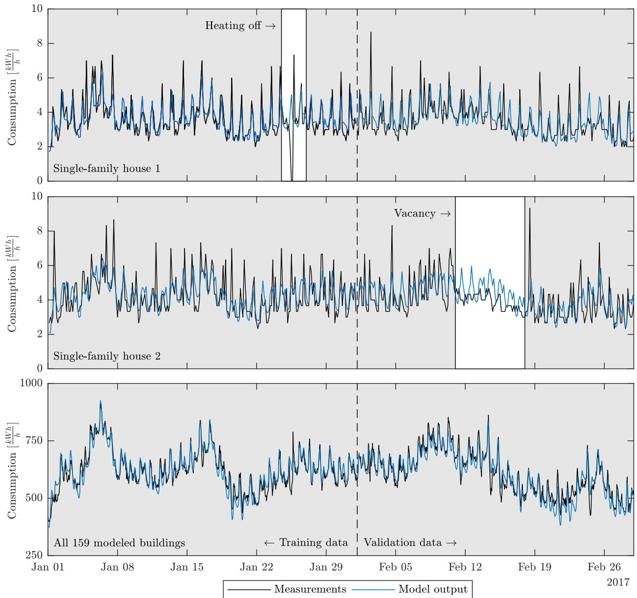
**Figure 2.** Comparison between measured consumption and model predictions. The top and middle graphs depict time series for two single-family houses, while the third depict the aggregated neighbourhood (159 single-family houses). The vertical dashed line separates the data used to calibrate the models (left side), and the data used for validation purposes (right side).
