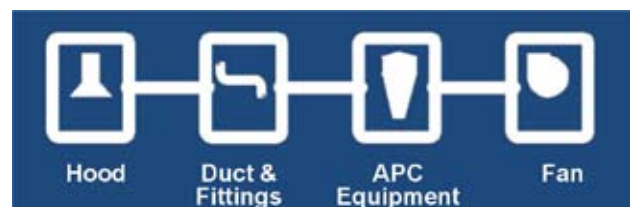
Figure 2. System design components.
