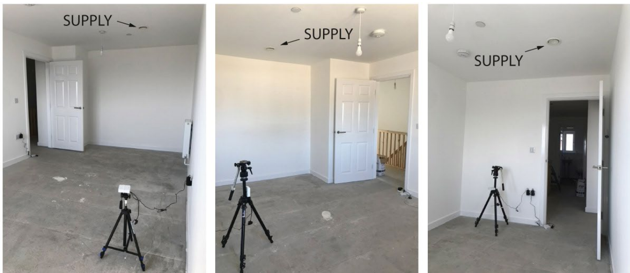
Figure 12. Tracer gas set-up in rooms of different sizes and layout.
