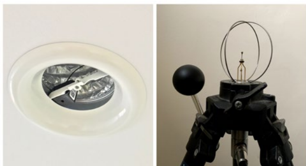
Figure 2. T/RH sensor in supply vent (left) and PMV experimental probe and sensor (right).
